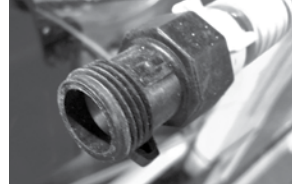
Unscrew the cap off of the connector, then screw your garden hose to the threads of the connector
